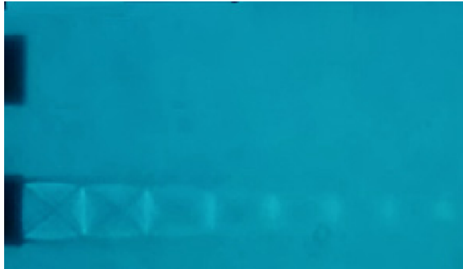
(a) Top nozzle NPR 0, bottom nozzle NPR 3
